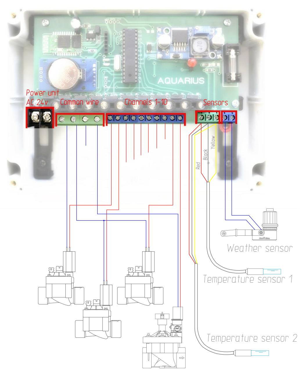
Up to 10 valves AC 24v one-time load of not more than 2A (for the included power supply)
